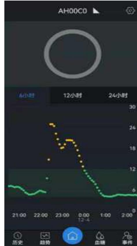
The transmitter is not attached tightly, and there is water vapor affecting the connector when taking a shower. In this case, the transmitter needs to be removed and reattached.
