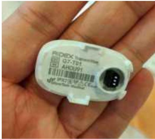
The 6-digit serial number of the transmitter must be entered correctly. If the serial number is occupied by others, contact the original user to unpair the transmitter or return it to the factory
