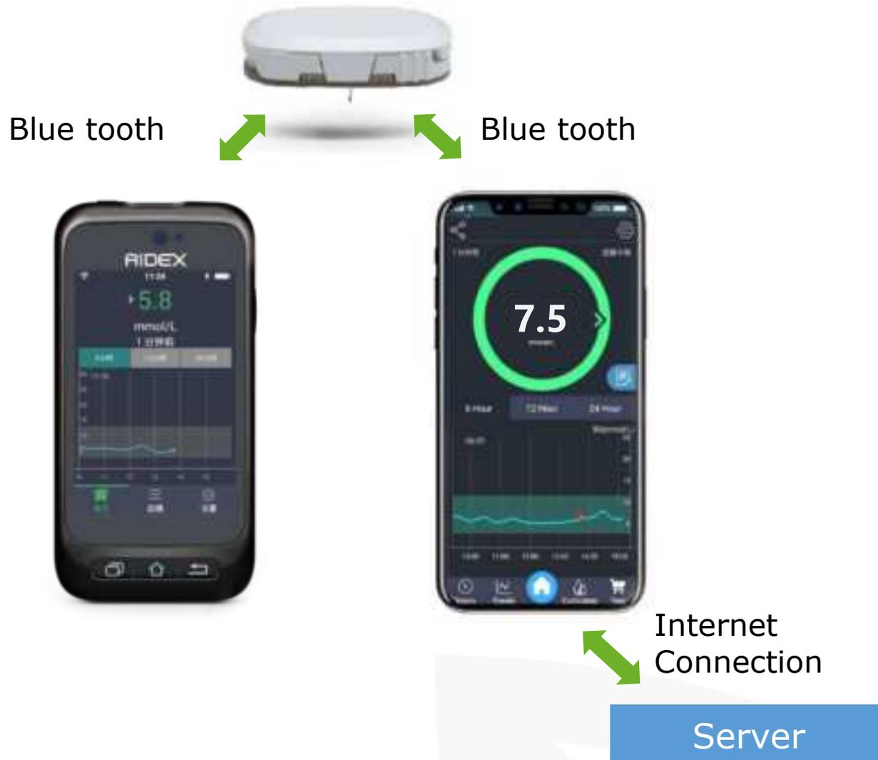
The transmitter **only stores the data of the sensor that was paired to it at the moment** and transmit the data via bluetooth to APP ,after the data was obtained by bluetooth,it will be uploaded to the server as long as the phone had internet connection ,which will be permanent memory. Users can download the AGP report based on the data from the server.
